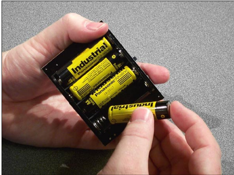
Figure A.2 - Installing batteries in the foundation.
