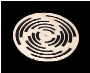
Figure 5.23 - A position encoding wheel for the Giant Music Box.
