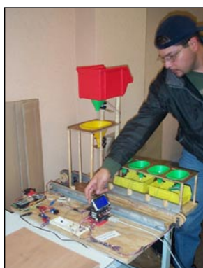
Figure 5.30 - The Livestock Feeding System, using an automated funnel to dispense grain to a number of simulated animal corrals.
