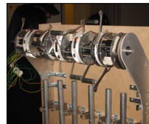
Figure 5.22 - A giant music box using a Tower to control hammers that would strike hollow sound pipes based on a predetermined note sequence.
