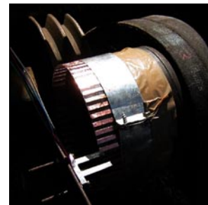
Figure 5.35 - The engine flywheel with copper strips attached for interrupting an optical sensor.
