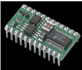
Figure 2.1 - The BASIC Stamp 2, a microcontroller module running a BASIC language interpreter.
