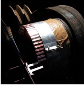
Figure 4.13 - The engine flywheel with copper strips attached for interrupting an optical sensor.
