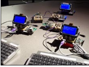
Figure 5.10 - A miniature instant-messaging application designed to teach kids about the ways in which individual nodes on networks communicate with each other both directly, and through central servers.
