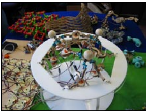
Figure 5.18 - A Topobo structure, built with a network of interconnected intelligent modules and capable of memorizing and playing back kinetic patterns.
